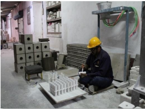
Slip cast finishing area – the ferrules are manually given finishing touches to remove any undulations or discoloration
