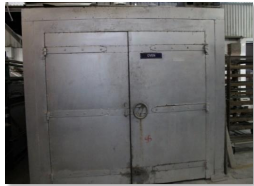
Gas oven – the bricks are dried in our gas oven before going for firing to remove the moisture
