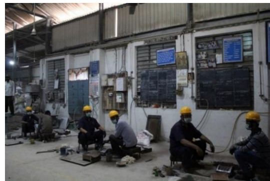
Moulding department – the moulds are checked for the dimension prior to sending for production. Intricate shaped bricks are hand moulded.
